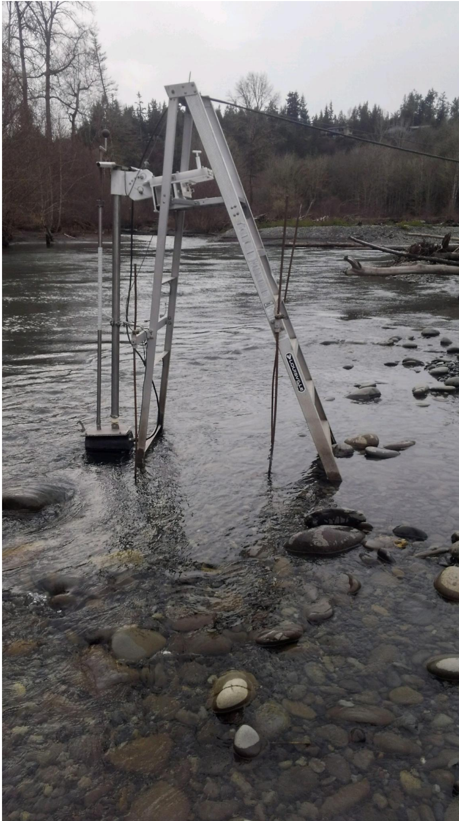
Figure 2. Photo of the HRC DIDSON site. Note low water that precluded fish passage up this channel during the majority of the coho run.
